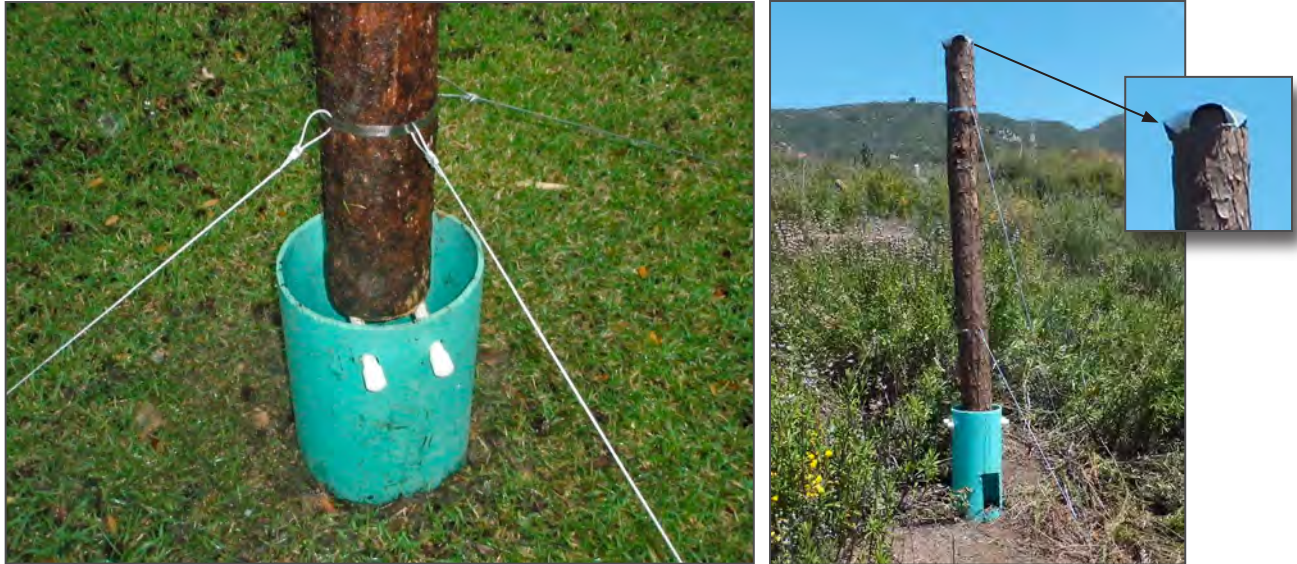
Figure 3—Vertical log suspended above ground (left), vertical log supported by steel cables capped with aluminum flashing (right).
