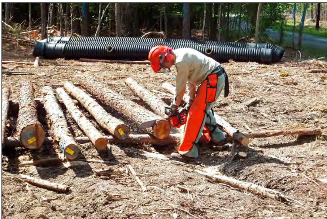
Figure 4—Voucher samples of the logs were collected from each log, tagged with the corresponding log number, and stored in the Santee Experimental Forest sample archive. Photo shows pine logs being processed at the Duke Forest.
