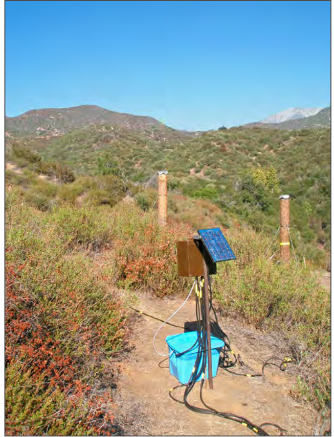
Figure 9—Datalogger monitoring powered by deep cell marine battery and solar panel (San Dimas).
